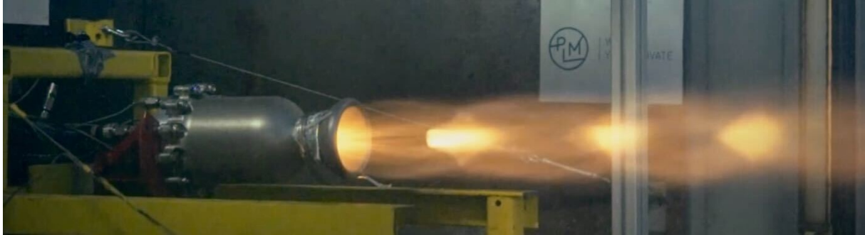
Figure 5: Combustion chamber during hot-fire testing
