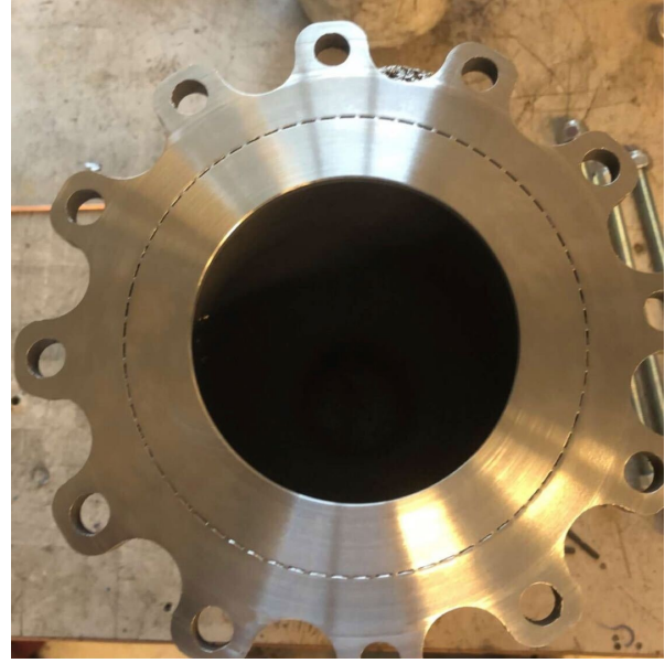
Figure 10: Mating surface of the combustion chamber, showing the circle of cooling channels.
