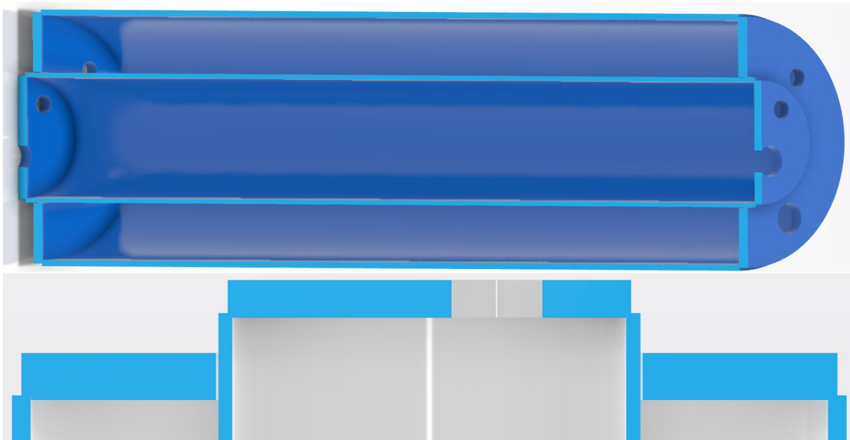
Figure 15: CAD of the coaxial propellant tank.
