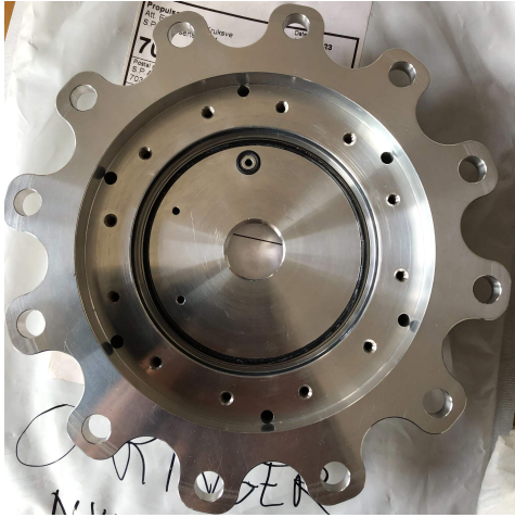
Figure 11: Bulkhead with O-rings.
