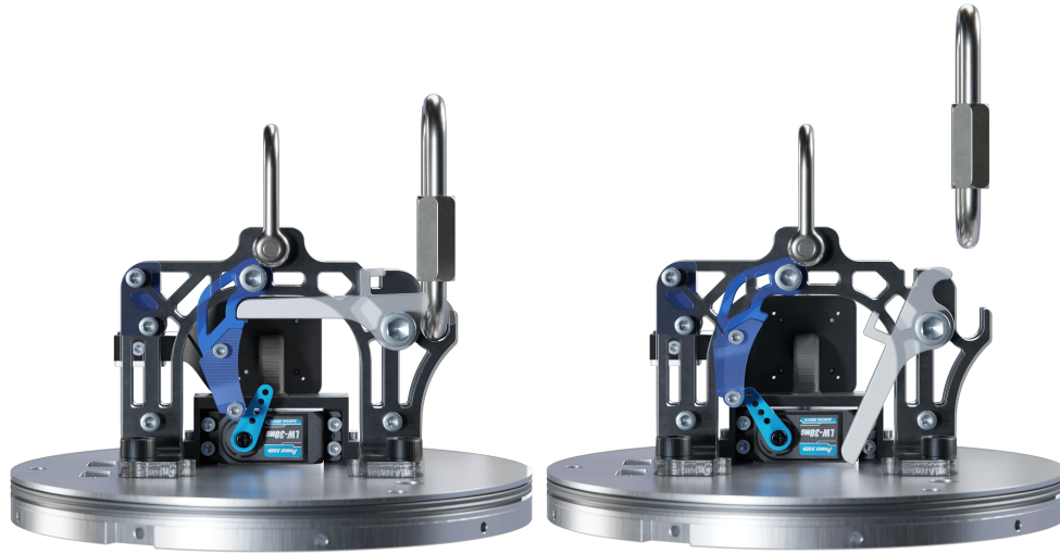
Figure 48: MCRS locked position (left), MCRS actuated (right). Note that one of the two servos is hidden to display the mechanism more clearly.
